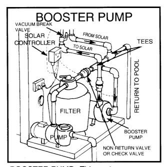
BOOSTER PUMP. This system removes load on pump and filter and can be made fully automatic by adding a solar controller - suitable for two story installation.
