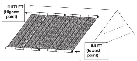
NOTE: The extra supplied parts are made in ABS and can be glued with PVC-glue. The headers (B) are made in PP (polypropylene) and CANNOT BE GLUED.
