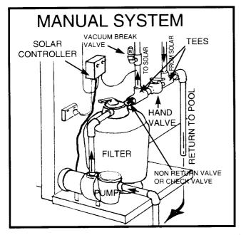
MANUAL system is operated by closing hand valve which diverts water to solar collector - this system must be cut in before any other pool equipment eg: gas heater, chlorinate. This system should be used on single story as it puts extra load on pump and filter (solar controller or time clock can be used to switch on and off.
